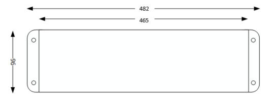
Fixing Holes M4 Product Height 60mm All Dimensions in mm Do not scale
